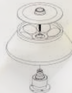
Single action of rotor coupling -Large volume Fixed Angle Rotor
